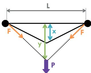
Minimum clearance =  $y + 1 \text{ m} + \text{fall arrester minimum clearance}$
